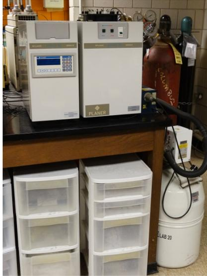
**Figure 2** - Planer Kryo 10 Series III Computer Controlled Cryogenic Freezer for sperm cryopreservation
