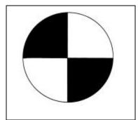
**Figure 1.** Diagrammatic view of a Secchi disk showing the light and dark pattern.
