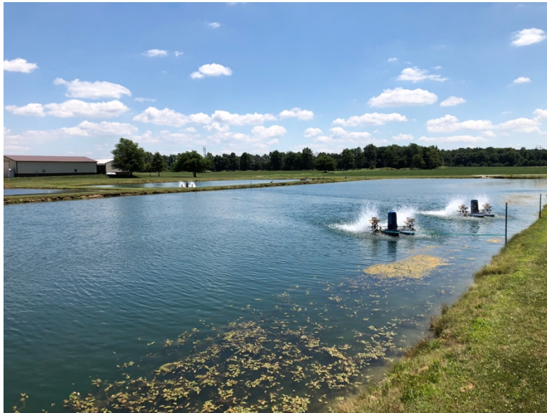
Figure 3. Intensive aeration (3.7 kW/ha; 2 hp/ac) at Millcreek Perch Farm LLC with the 0.40 ha pond in the foreground and the 0.20 ha pond in the background. Paddlewheels ran 24/7 for the duration of the project.
