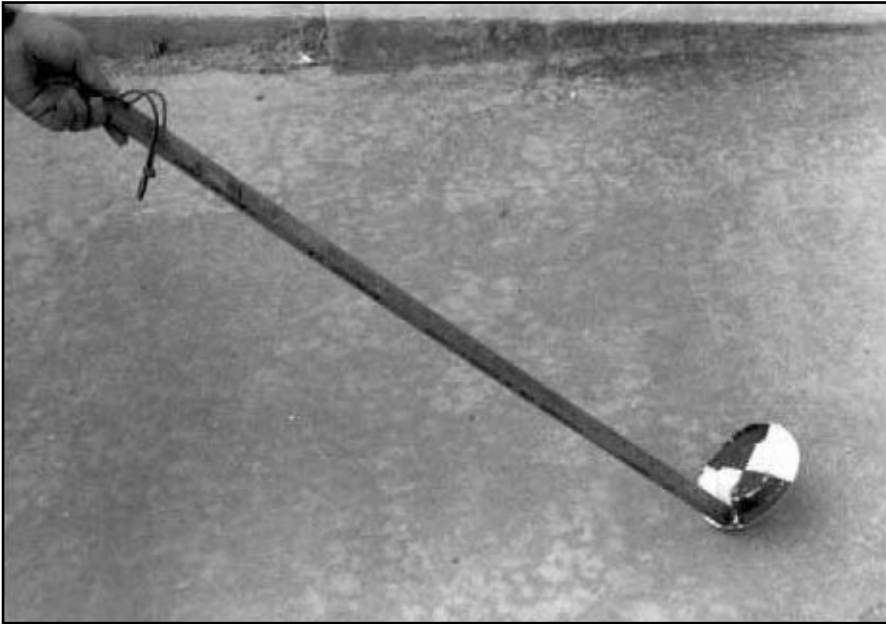
Figure 1. Secchi disk for evaluating pond blooms.
