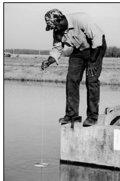
Figure 5. A Secchi disk is a 6- to 8-inch disk of painted wood or plastic, often with alternating white and black quadrants. The disk is fastened to a yardstick or calibrated string. To measure the secchi disk visibility, the disk is lowered into the water until it disappears from view, and the depth recorded. The disk is then raised until it reappears. The depth is again recorded. The average of the two readings is called the secchi disk measurement. The secchi disk cannot be used in muddy ponds, as it will measure mud turbidity rather than plankton abundance.
