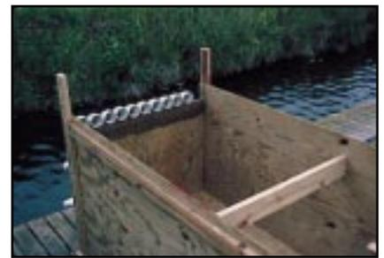
*Figure 2. IPR (out of the water) showing position of air-lift system and eddy board.*
