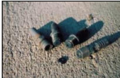
Figure 5a. PVC tubing connectors with restriction orifice(s).
