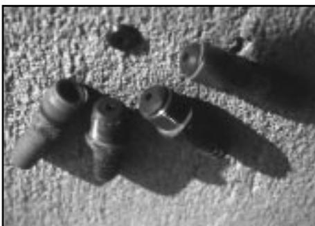
Fig. 7. PVC tubing connectors with constriction orifice.
