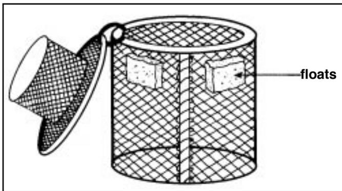
Fig. 2. The 4' x 4' cylindrical cage design.
